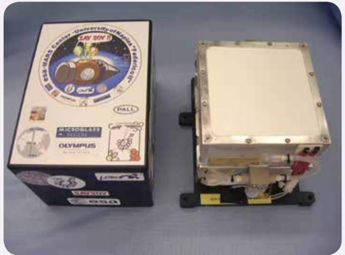
Figure 6 - Flight hardware of the SAYSOY (Space Apparatus to Yield SOY sprouts) ESA project: germination chamber (upper module), hydraulic system (middle level), and electronic system (basal module). The experiment was performed to investigate the possibility of producing soy sprouts onboard to integrate a crew's diet during long-term missions and/or permanence on space stations, and conducted successfully by the team of prof. Veronica De Micco and Giovanna Aronne of the Department of Agricultural Sciences of the University of Naples Federico II, during the Foton-M2 campaign (31 May 2005 through 16 June 2005).
