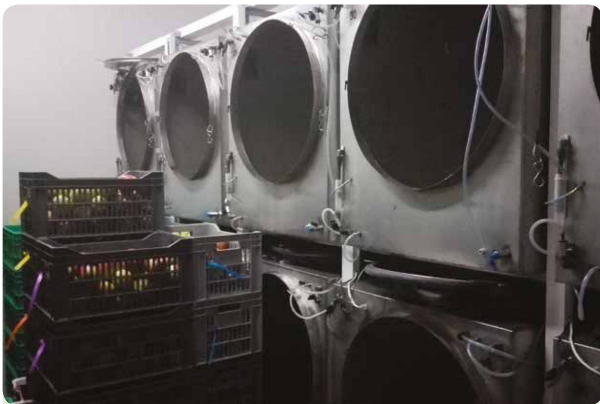
Figure 2 – Storage chambers to study the effect of controlled and modified atmosphere on fruit quality.
