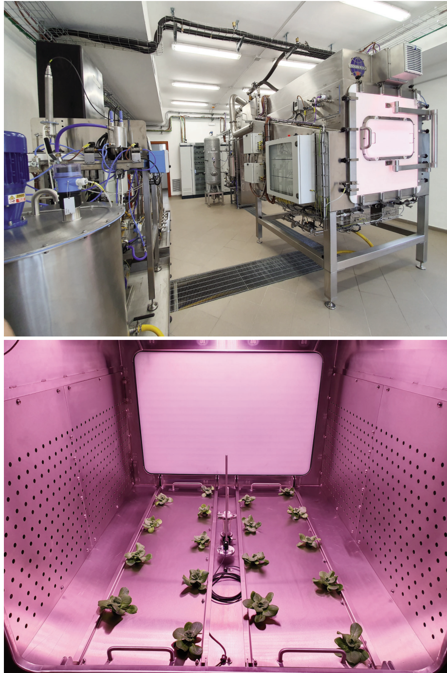
Figure 6. General view of the laboratory devoted to Space research on higher plants at the University of Naples (Italy) and an internal view of the Plant Characterization Unit (PCU) (Credits Antonio Pannico).
