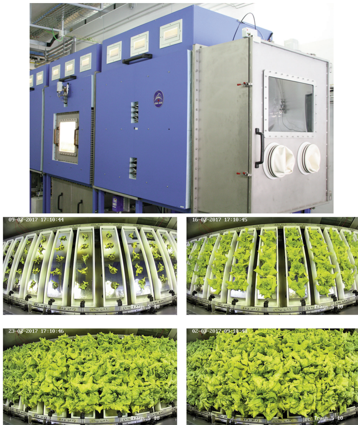
Figure 5. Higher plant chamber (HPC) of the MELiSSA pilot plant (external and internal view) at the University of Barcelona (Spain) and lettuce plants in subsequent stages of development during the ACSA experiments.
